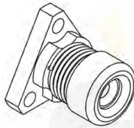
Size 8 (20mm) and Size 11 (28mm) anti-backlash nut
